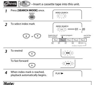
The time gap between index marks should be more than 1 minute for SP
